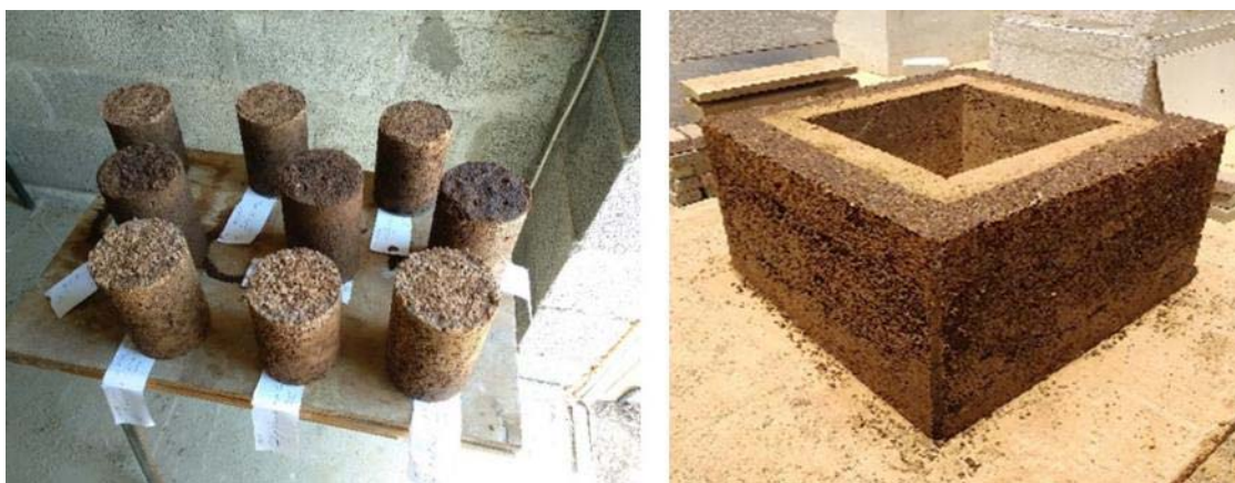
Figure 6: (left) OP biocomposite samples with varying OP particle size, water content, and binder ratio; (right) test cell walls, with respective 10 cm-thick layers of external orange peel (OP) biocomposite insulation and internal rammed earth (RE) mass, before plastering and roof installation.
