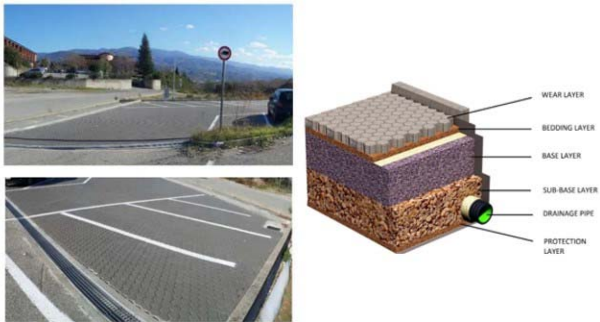
Figure 9: The permeable pavement experimental site at University of Calabria.
