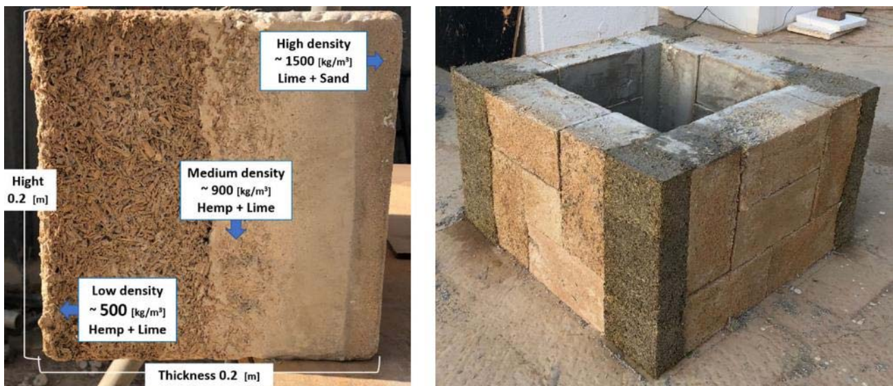
Figure 4. (left) Gradient HL cross section; and (right) gradient HL test cell before plastering and roof installation, with homogenous hemp-lime cast on the corners to prevent thermal bridges.
