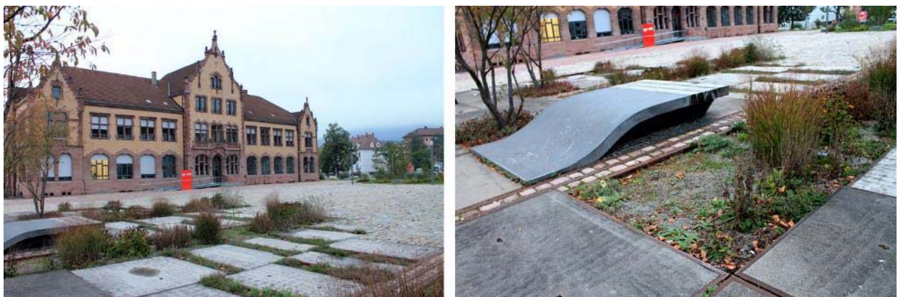
Figure 11: Local planting and view to the old train station of Freiburg. The details of the train tracks and the memory of the area is brought back in a system showing applicability of circular city material recycling applications (left), and details of seating designed as being peeled-off the ground to allow for maximizing the space for permeable green surfaces that are entry points to the infiltration system to the underground storage, but also to the groundwater reservoir (right).
