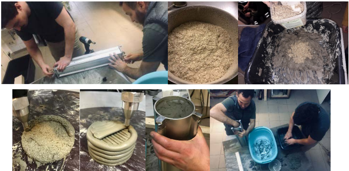
Figure 2. Preparation for each printed trial, from upper-left clockwise: taking apart for cleaning, measuring materials (shredded hemp hurds), mixing, loading the cartridge and printing trials of mixes with hemp fraction of 0% (no hemp) and 6%, respectively.
