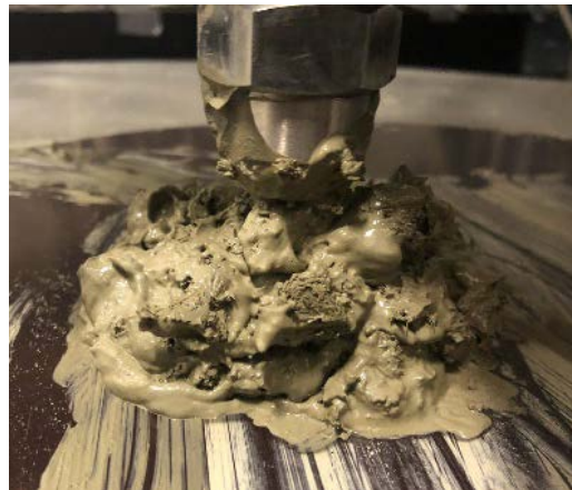
Figure 5. Unsuccessful printing trial with hemp content of 10% by mass.
