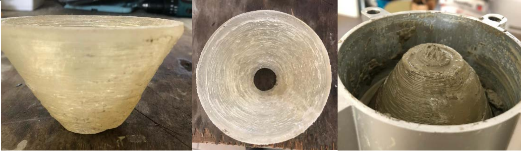
Figure 3. 3D printed plastic cone as a solution to better direct the flow of the mix from the cartridge to the extruder
