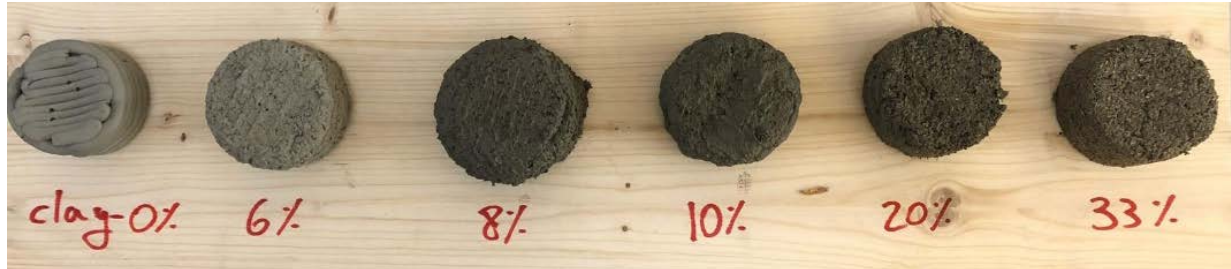
Figure 4. 3D printed and handmade hemp-clay samples with varying fraction of hemp in the clay. ; mixes with 0-10% hemp were printed, while mixes with 20% and 33% hemp were made by hand.
