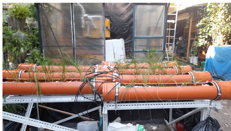
Figure 2. The lab-scale vertECO© raft system used in the experiment
